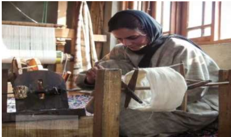
Fig.2: Spinning of Wool
