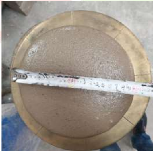
Figure 2: Flow table test for the fresh mix.
