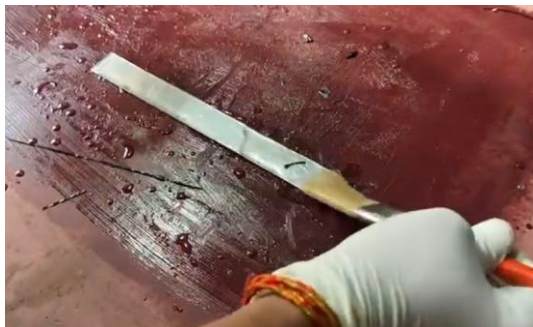
Fig. 26 Resin application on Specimen
