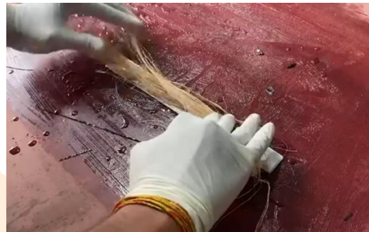
Fig. 27 Sisal Fiber layup on specimen
