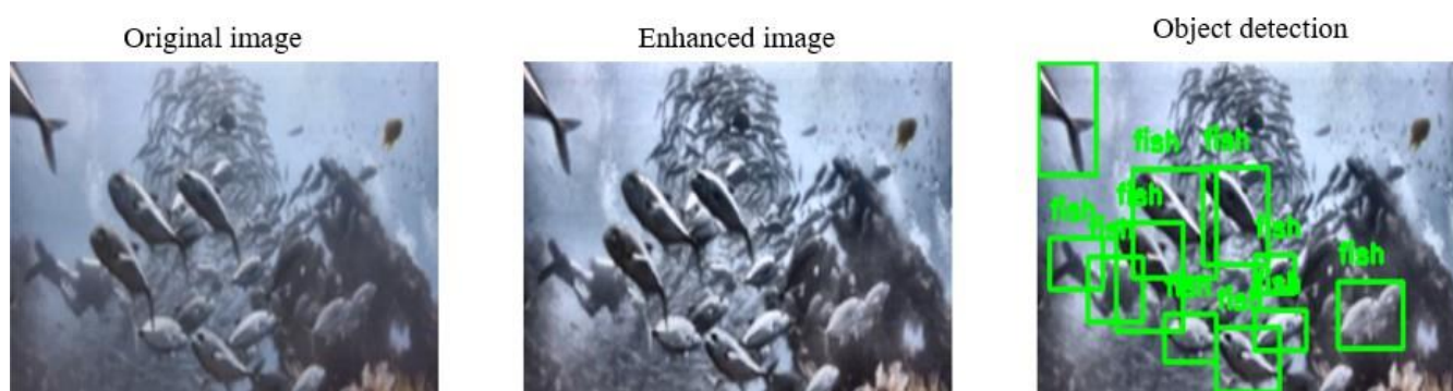
Fig. 9. Image enhancement and object detection using multi color space residual network, swin transformer and YOLO V8
