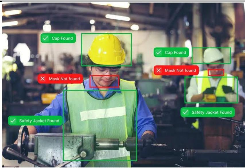
Visual inspection of results showed that the system accurately identified multiple workers simultaneously and correctly distinguished between workers with and without required safety gear. Bounding boxes were clearly drawn around each detected PPE item with corresponding confidence scores, providing clear visualization for monitoring purposes. In cases where PPE was missing, the rule-based compliance mechanism successfully triggered alerts, ensuring immediate attention to safety violations.
