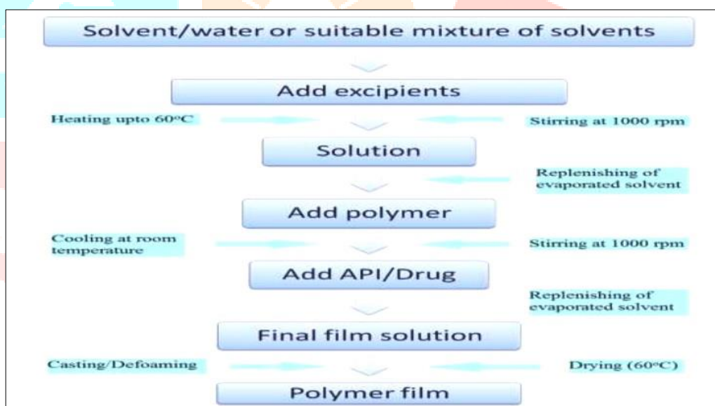
Figure no: 2 Solvent casting method flow chart
