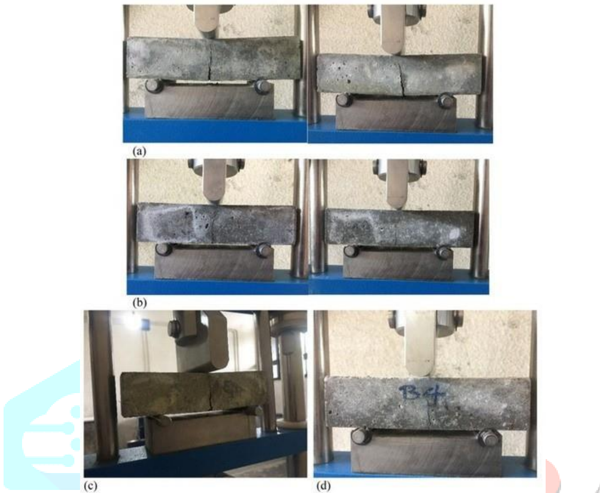
Figure 12. Failure of flexural samples: (a) mixture of 'F'; (b) mixture of 'CF1'; (c) mixture of 'CF2'; (d) mixture of 'CF3'.
