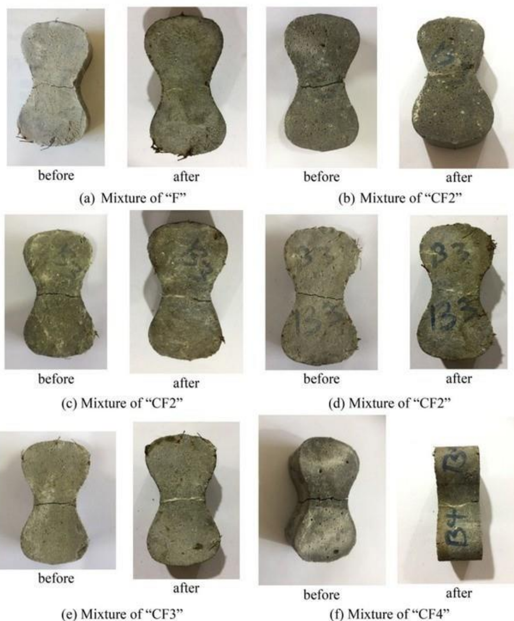
Figure 13. Crack sealing in direct tension samples after the healing period.
