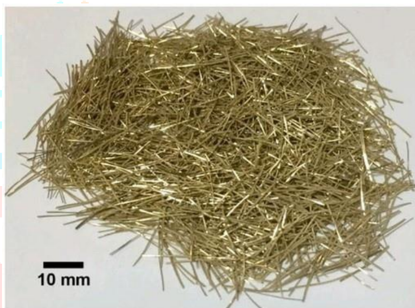
Figure 1. Micro steel fibers used in the present study.
