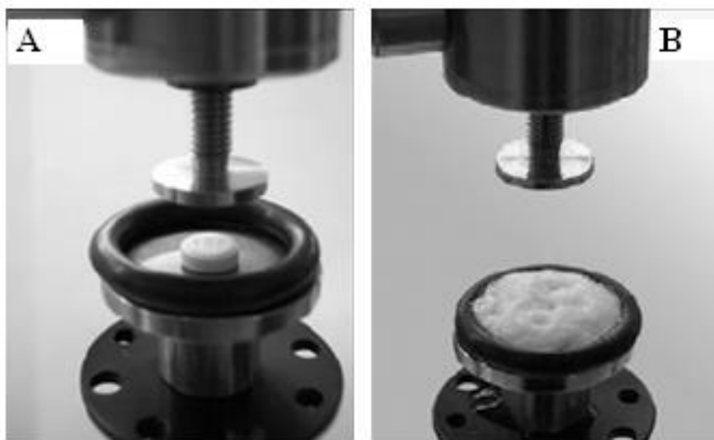
Fig. 8 ElectroForce® apparatus for Disintegration test A. OODT mounted on test plate before loading. B. OODT after completion of Disintegration test
