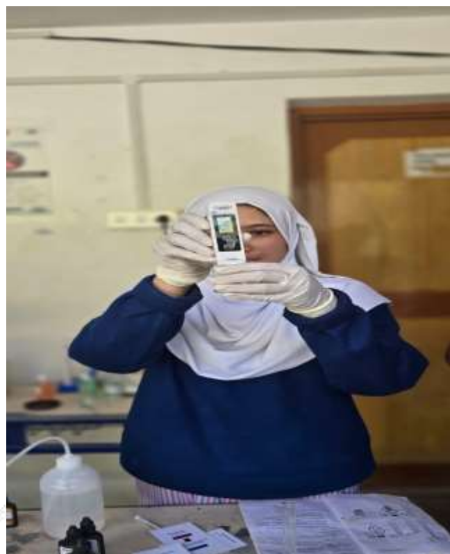
Figure 1.4. To determine the TDS and electric conductivity of sani water.
