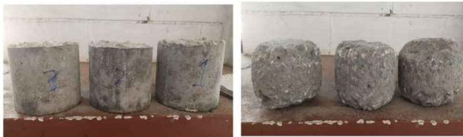
Figure 9: Specimen forms during the 0 and 300 RPM Cantabro loss tests
