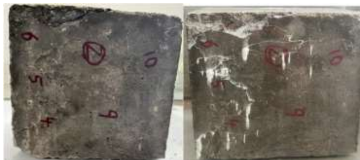
Figure 7: The ability of self-healing bacterial concrete to repair cracks on days 1 and 7
