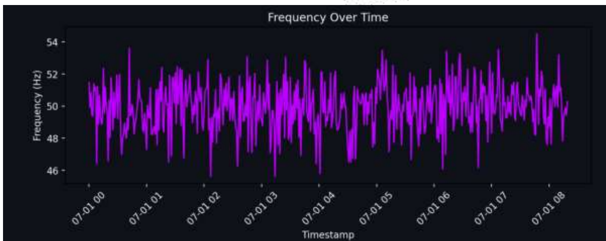
Figure 4: Frequency variation over time - Visualization of frequency data (in hertz) across different timestamps, highlighting fluctuations that could indicate instability in power supply
