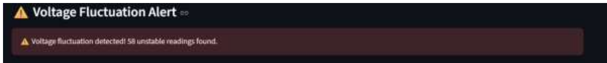
Figure 5: Fluctuation Alert System -Automatic alert is generated when unstable voltage readings exceed the defined threshold, providing early warning to users
