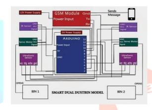
fig 1 connections of arudino board
