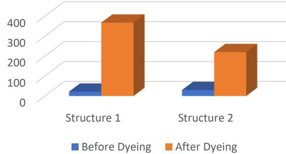
According to the test results, it is clear that both structure 1 and structure 2 experience a sudden rise in UV protecting properties after dyeing. This improvement guards the sportsmen and also active individuals who spend long hours outdoors against the deforming UV radiation emitted by the sun. The process of dyeing have stronger influence on structure 1 compared to structure 2, and hence sample 1 provide better competitiveness in clothes that are for outdoor use.
