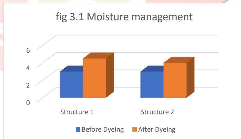
According to the test results, it is evident that both Sample 1 and Sample 2 acquired moisture management properties upon dyeing. This improvement in moisture management properties enhances quick drying and wicks sweat from the skin, leaving the wearer feeling comfortable. Sample 1 performed better in terms of moisture management than Sample 2. This is especially true in high-intensity sportswear, where the ability to keep the body dry reduces discomfort while increasing athletic performance.
