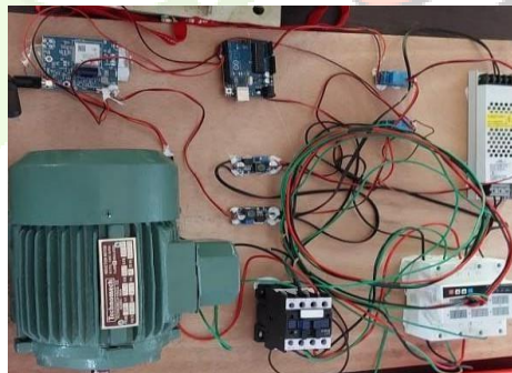
Figure 2: Working Prototype of Pump Control Unit for Smart Farming
