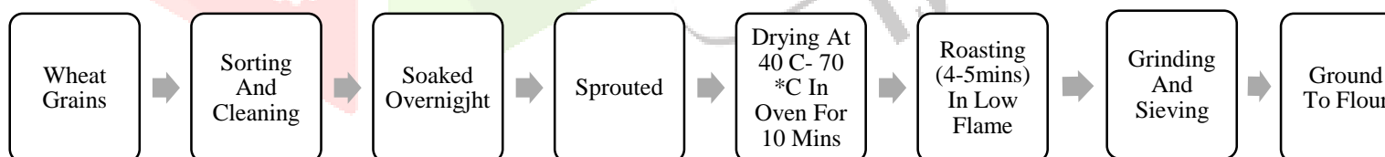
(figure 03) flowchart of preparation of sprouted wheat flour
