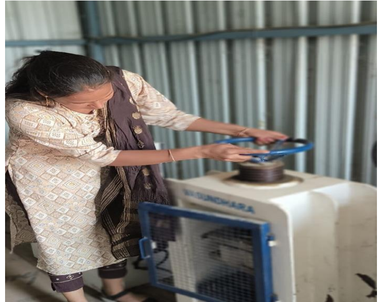
Figure 3 - Compressive strength testing on CTM
