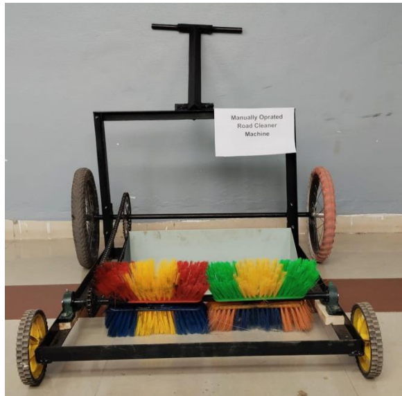
Fig.3.1 Design of eco-friendly road Cleaner machine
