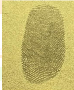
Fig 5: latent fingerprints developed on chart paper.
