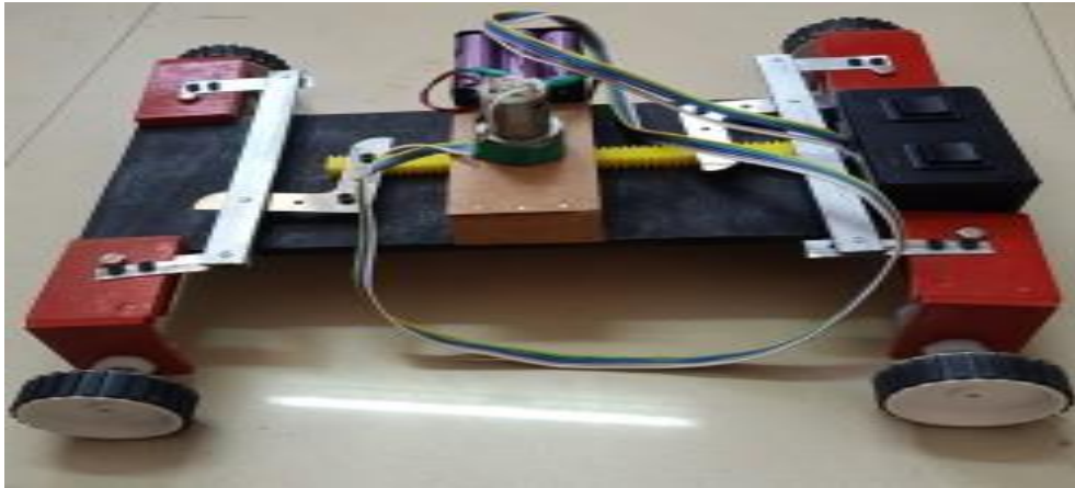
Fig.: (A) Four-Wheel Steering Linkage System”
