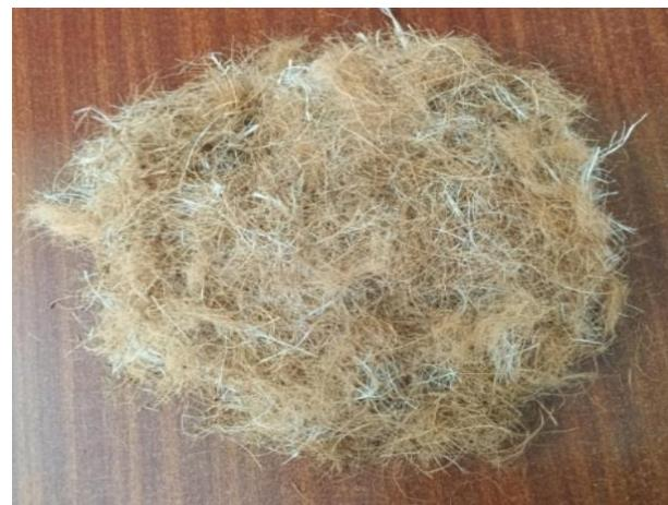
achieve the needed strength, inflexibility, and humidity retention. The coconut coir is first washed and cut into invariant pieces. The banana filaments are also removed from the factory, washed, and dried so that they can be fluently mixed. Both the filaments are also mixed together unevenly. This mix takes the advantage of both — banana fiber provides strength, and coconut coir retains humidity.
