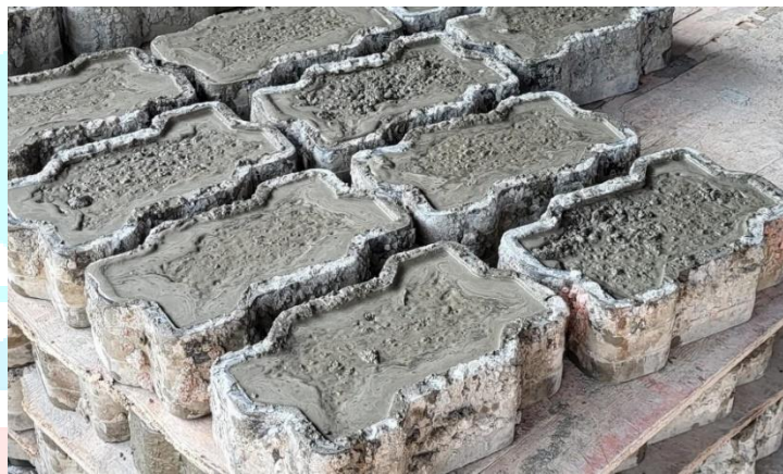
Fig.7 Manufacturing of Interlocking Tiles.
