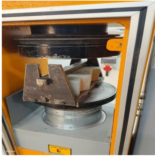
Fig.9 Split Tensile Strength on Interlocking Tiles.
