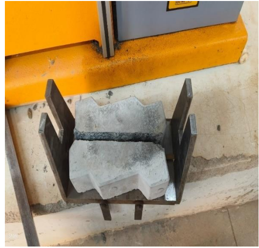
Fig.9 Split Tensile Strength on Interlocking Tiles.
