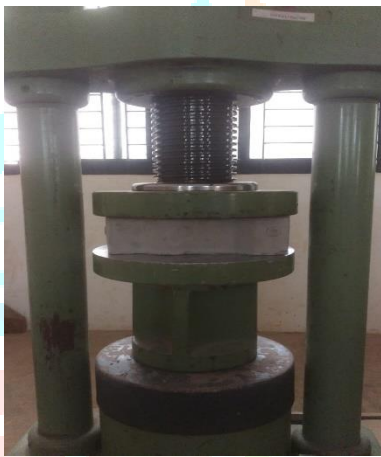
Fig.8 Compressive Strength Test on Interlocking Tiles.
