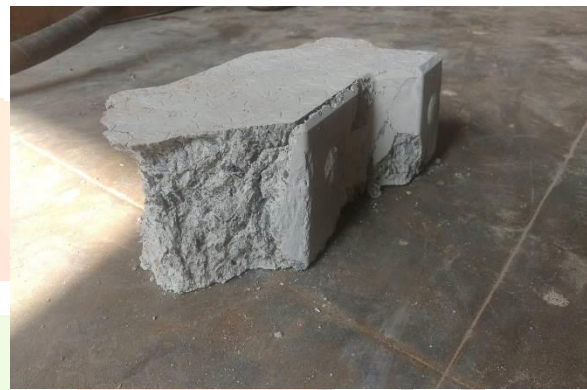
Fig.8 Compressive Strength Test on Interlocking Tiles.
