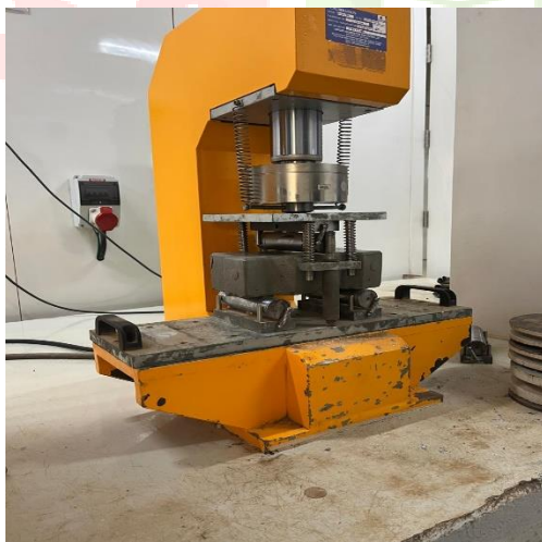
Fig.10 Flexural Strength Test on Interlocking Tiles.
