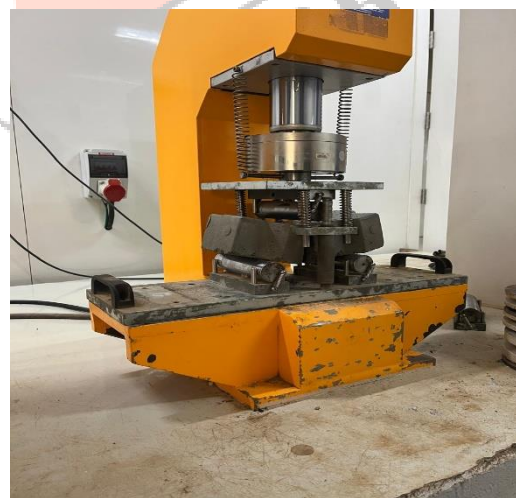
Fig.10 Flexural Strength Test on Interlocking Tiles.
