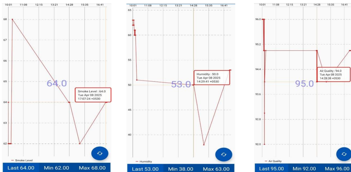
Fig-10: Results of Smoke Level, Humidity and Air Quality
