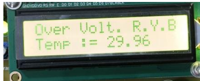
Figure 3. Over voltage fault detection on LCD display
