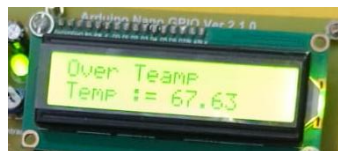
Figure 5. Over temperature fault detection on LCD display
