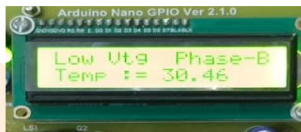
Figure 7. Single phasing fault detection on LCD display
