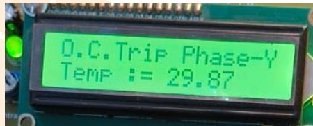
Figure 4. Over current fault detection on LCD display
