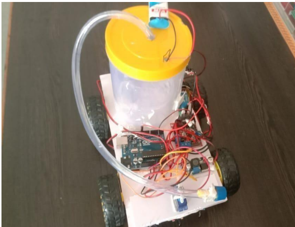
Fig. 7: Model of Fire Extinguisher Robot
