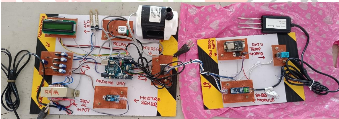
Fig. 4: The image shows a smart irrigation system deployed in an outdoor environment, integrating sensors, an Arduino-based controller, and an automated water management setup.
