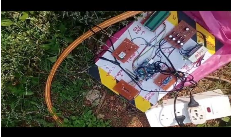
Fig .3: The image displays a complete smart irrigation and soil monitoring system integrating Arduino UNO, NodeMCU, multiple sensors, and an automated water pump for precision agriculture.
