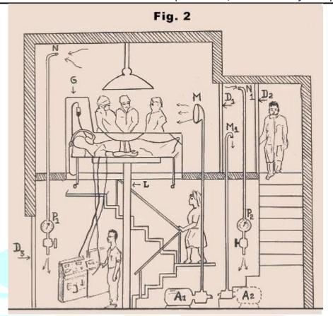
In Fig. 2, the doctors and the exposed part of the patient are placed in a space having pressure equal to the sum of atmospheric pressure and blood pressure of the exposed part of the patient while the patient is lying under normal atmospheric pressure.
