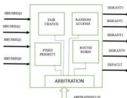
Fig5. Functional diagram of AHB Arbiter
