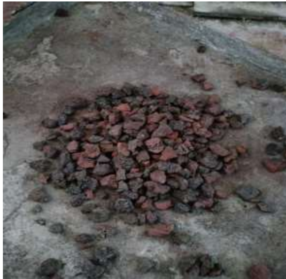
Figure No. 05 Overburnt Brick pieces
