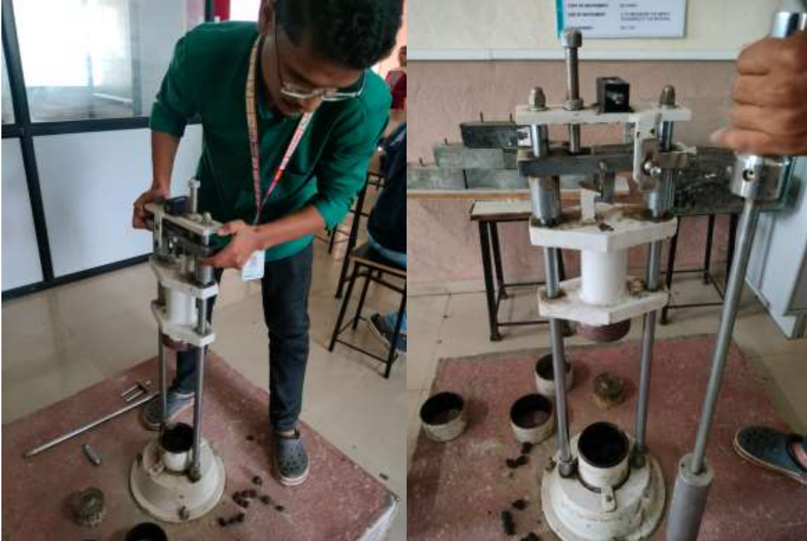
Figure No. 09 Impact aggregate test
