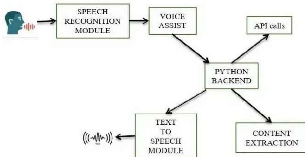
The architecture presents a modular approach to building a VVA system. It consists of distinct components responsible for handling different aspects of voice interaction and task fulfillment. The flow generally starts with speech input, moves through processing and understanding, and concludes with generating and delivering a response.
