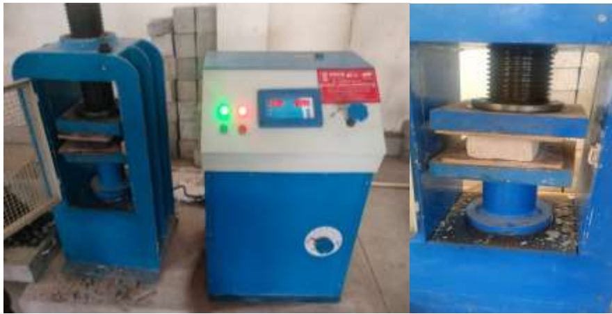
Figure 2 Compressive strength test of fly ash brick
