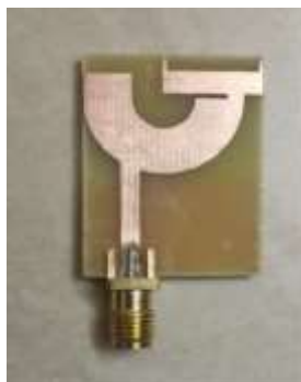
Fig.7. Fabricated UWB Monopole Antenna
