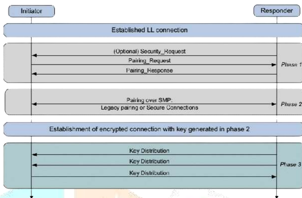
Figure 3. A visual representation depicting the fundamental process of Bluetooth Low Energy (BLE) pairing (Ren, 2016)
