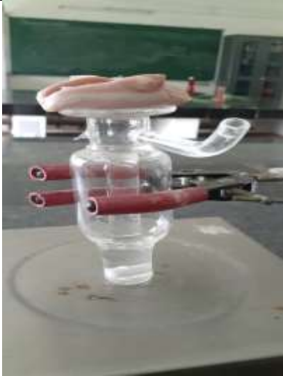
Fig 4: Ex Vivo Permeation Using Goat Tongue
