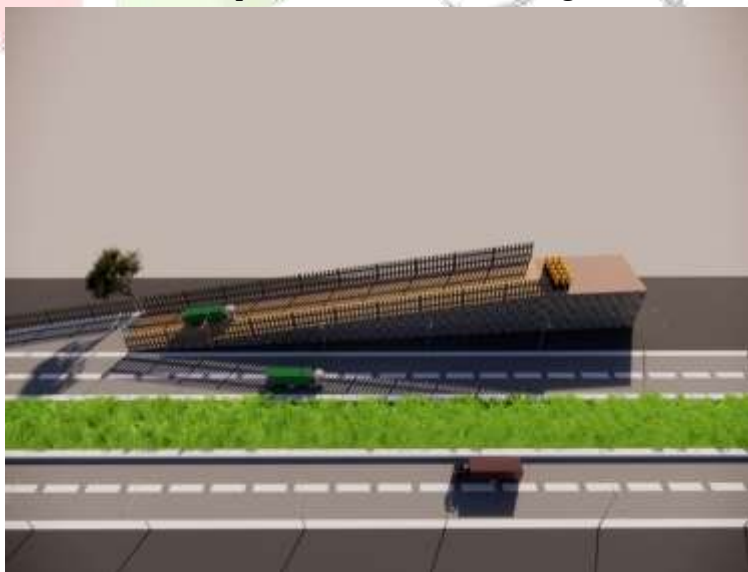
Figure 2. Emergency Escape Ramp on Samruddhi Mahamarg
