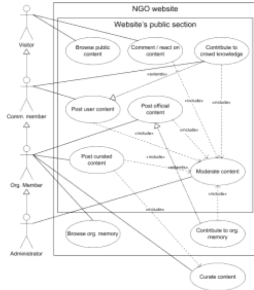
Fig. 2. UML case diagram of stage 2. Here “Comm. meber” is a registered user with “creative permissions”, able to contribute to SKE.
