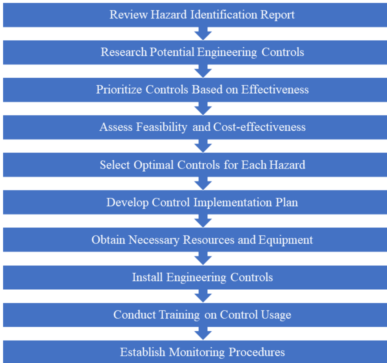
Fig.2.Process of selecting and implementing engineering controls to mitigate identified hazards in the MDV weld shop.
