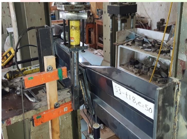
Figure 7: Typical Failure mode of the tested beams
