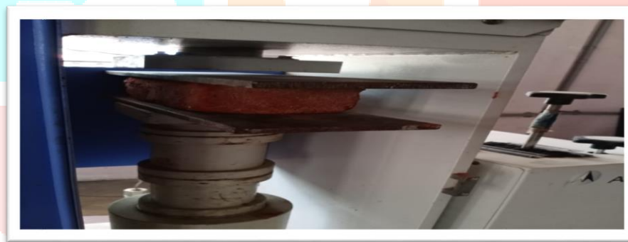
Fig.9 normal brick at failure point
