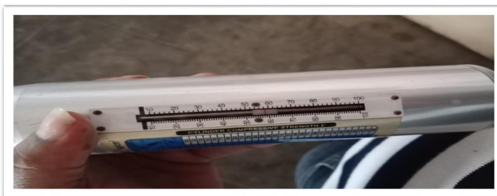
Fig.8 Rebound number for plastic brick
