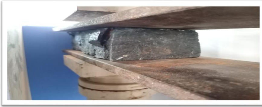
Fig.10 At plastic brick failure point
