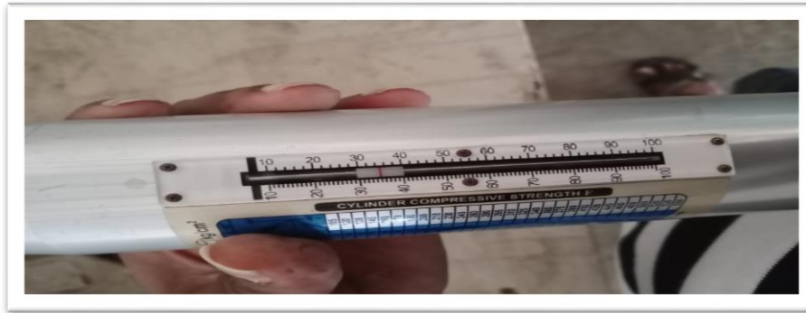
Fig.7 Rebound number for normal brick
