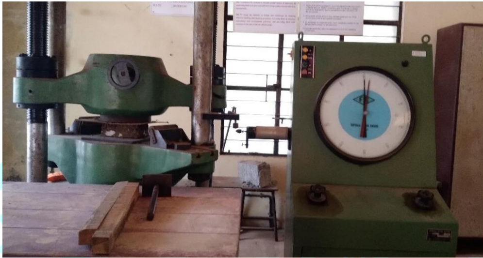
Fig 5.9: Compressive strength testing in Universal Testing Machine
