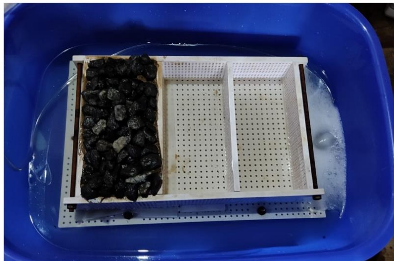
Fig 5.8: Batch reactor along with aggregates getting manufactured for 7 th day test, provided with an additional loading on top.
