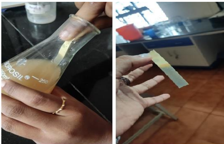
Fig 3.2: Testing the pH of cementation media using litmus paper
