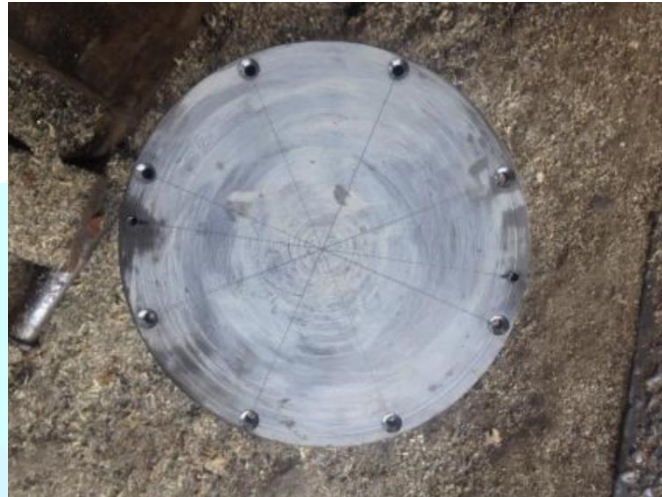
Fig. 4. Disc for wear resistance test.
