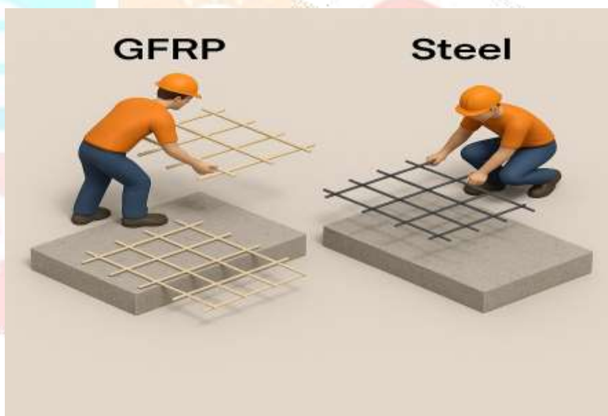
Figure 3: 3D schematic representation of reinforcement placement for GFRP and steel in rigid pavement slabs highlighting differences in handling and cover detailing
