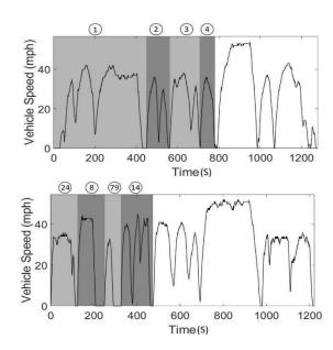
Fig. 1. The first four segments of a sample real duty cycle (top). A sample synthetic duty cycle created by concatenating segments 24, 8, 79, and 14 from the real data (bottom)
