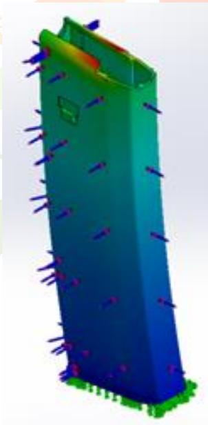
Fig 7: Displacement Analysis of AISI 1020 Magazine at -57 °C
