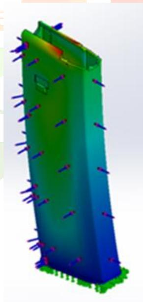
Fig 5: Displacement Analysis of Nylon 6,6 with 10% fibre glass Magazine at -57°C
