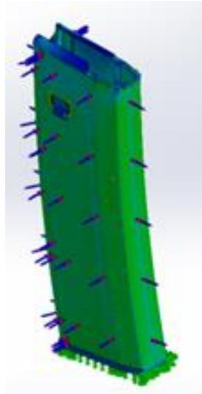
Fig 4: Stress Analysis of Nylon 6,6 with 10% fibre glass Magazine at -57°C
