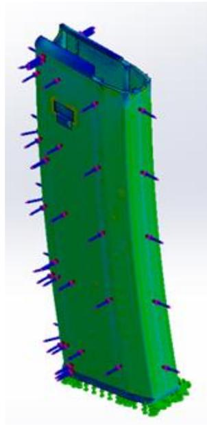
Fig 6: Stress Analysis of AISI 1020 Magazine at -57 °C
