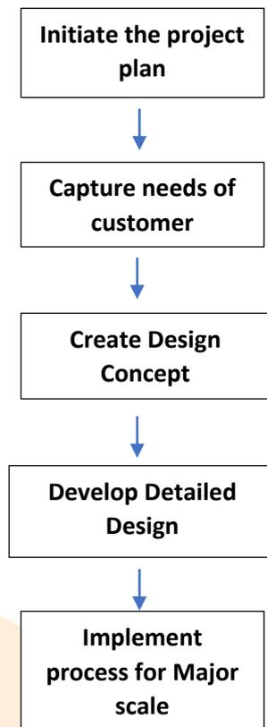
**Figure 1 - 5 step process of DFSS**
