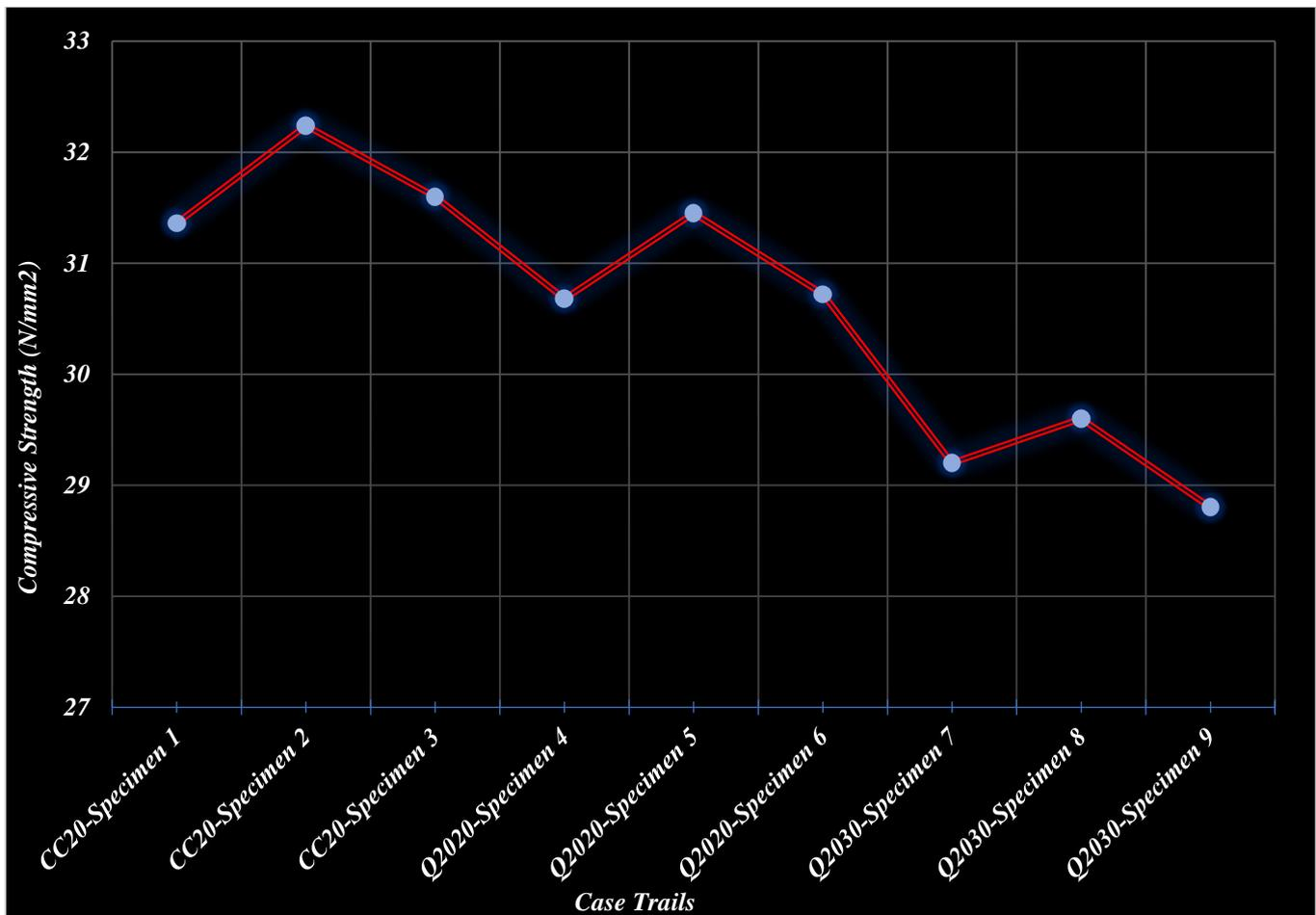
Fig. 2 Compressive Strength for Case Trials for M20 concrete
