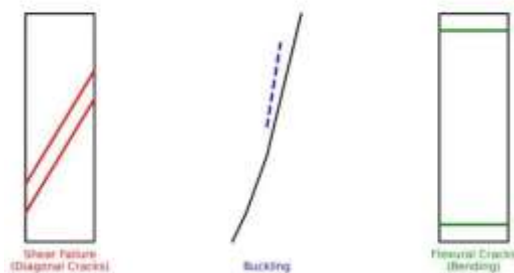
Figure 2.1 Typical Column Failures under Earthquake
