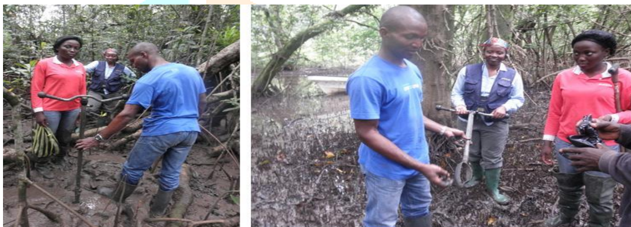
Plate 2: Collection of soil at different depths with a soil Auger in Avicennia stand in Cameroon
