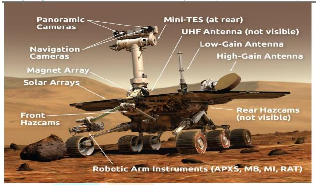
Capturing and filtering magnets The Capture and Filter magnets are located in the front of the rovers. The three instruments on the Instrument Deployment Device will study it once enough dust has been attracted to the magnets.
