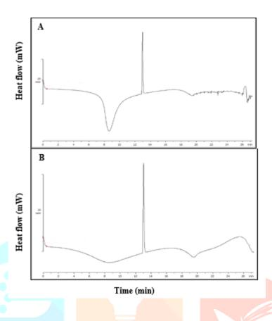
Figure 2. DSC thermogram of (A) mung bean protein isolate and (B) soy bean protein isolate
