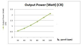
The output power with cotton rope power amplifier is seen to increase with the increase in input speed, as the power handling capacity of amplifier is seen to increase with the increase in input speed and maximum torque of 2.12 watt is observed at speed of 100 rpm
