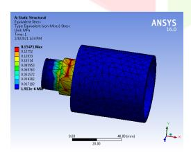
The maximum Von-misses stresses in the part are 0.1571MPa which is far below the allowable stress hence the part is safe
