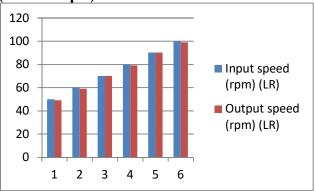
The input and output speeds with cotton rope power amplifier are seen to be same with negligible difference on account that the input and output shafts are connected via the cotton rope through the input and output arms
