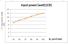
The input power with cotton rope power amplifier is seen to increase with the increase in input speed, as the voltage and current are both increased by the supply side.
