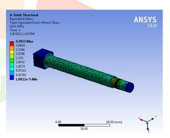
The maximum Von-misses stresses in the part are 4.282 MPa which is far below the allowable value hence the part is safe
