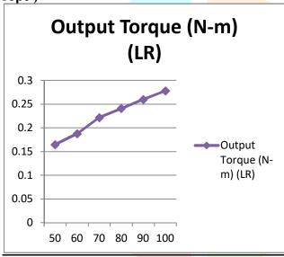
The output torque with cotton rope power amplifier is seen to increase with the increase in input speed , as the power handling capacity of amplifier is seen to increase with the increase in input speed and maximum torque of 0.206~N-m is observed at speed of 100~rpm
