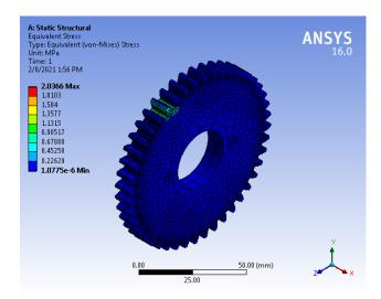
The maximum Von-misses stresses in the part are 2.036 MPa which is far below the allowable value hence the part is safe
